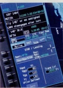
The Apex displays include a primary flight display (PFD, left) with adjoining engine information and navcom tuning functions. A flight plan page on the MFD (below, left) is navigated with a joystick, and allows the pilot to select preflight, takeoff, and descent pages. The caution, warning, and system status displays (below) are at the left side of the lower multifunction display.
